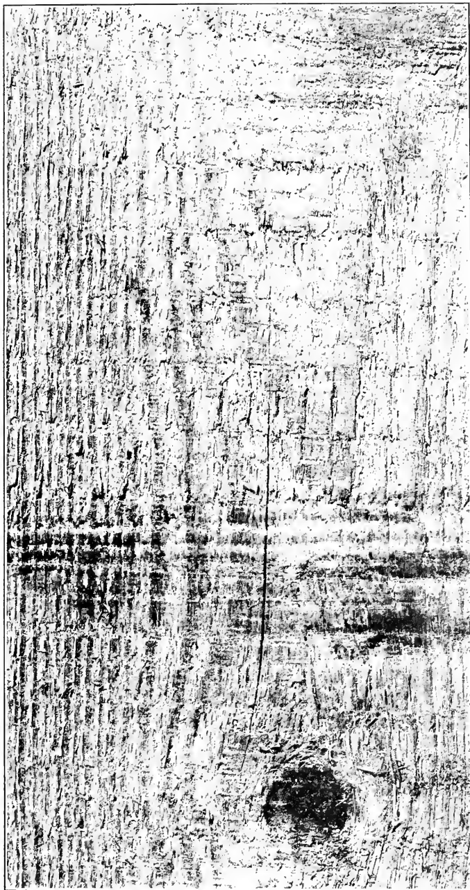
A check in 1 by 6 inch lumber resulting from the uneven drying caused by an excessively wide sticker. Narrow stickers, from 1\frac{1}{4} to 2 inches in width, permit better drying of the wood they cover
